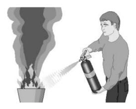
Extinguishers are classed by the type fire they can put out. Some extinguishers are **Combination** types that can be used on several different types of fires
